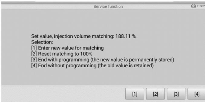
**Figure 5-24 Sample Injection Rate Screen**
