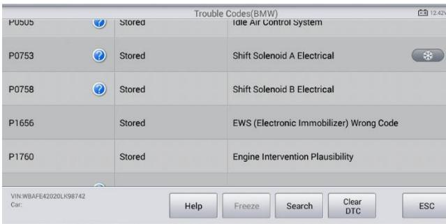
**Figure 4-19 Sample DTC & FFD Screen**
