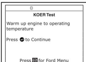
5. When prompted, turn off all vehicle accessories, turn ignition key OFF and wait for the on screen prompt. If you wish to exit the KOER test at this time, press the **SYSTEM MENU**
