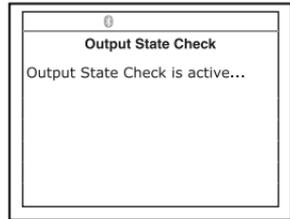
10. When prompted, press the accelerator pedal once, then release. This activates the Output State Check and energizes most of the actuators (relays and solenoids) that are controlled by the vehicle's computer.
