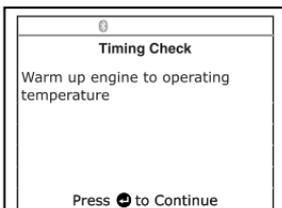
6. When prompted, turn off all vehicle accessories, turn ignition key OFF and wait for the on screen prompt. If you wish to exit the Timing Check procedure at this time, press the **SYSTEM MENU**
