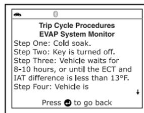
7. When you are finished viewing the Trip Cycle Procedures, press the **ENTER ↵** button to return to the Trip Cycle Procedures menu, or, press the **M** button to return to the Main Menu.
