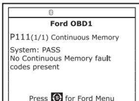
10. If more than one code was retrieved, press **DTC** button, as necessary, to display additional codes one at a time.
