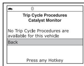
6. The Trip Cycle Procedure screen shows the specific set of operating procedures that ensure the vehicle is driven in such a way that all the required "Enabling Criteria" for the Monitor to run and complete its diagnostic testing are met. Use the **UP ▲** and **DOWN ▼** buttons, as necessary, to view the entire screen.
