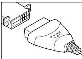
3. Connect the Diagnostic Tool cable connector to the vehicle's DLC. The cable connector is keyed and will only fit one way.
