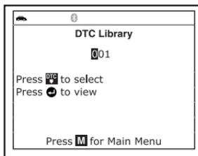
5. Select the remaining digits in the DTC in the same way, pressing the **DTC** button to confirm each digit. When you have selected all the DTC digits, press the **ENTER ↵** button to view the DTC definition.
