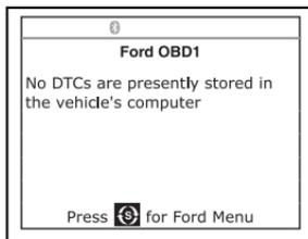
10. If no problems are found during the KOER Self-Test, the computer sends a "PASS code" (code 11 or 111) to the Diagnostic Tool. Code 11 or 111 indicates that all the relays and actuators and their related circuits that were tested during the KOER Self-Test are OK, and no faults were found.
