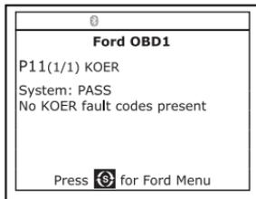
11. After the Diagnostic Tool retrieves all the KOER Self-Test DTCs, turn the engine off, and disconnect the Diagnostic Tool from the vehicle's test connectors. The DTCs retrieved are now stored in the Diagnostic Tool's memory.
