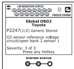
13. If more than one DTC was retrieved, press and release the **DTC** button, as necessary.
